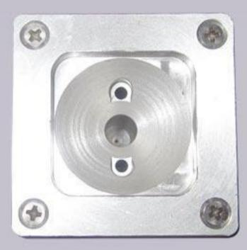
The clean-out opening of the drop-tube can make both the interior and exterior wall of the drop-tube cleaned and avoid the cross pollution.
