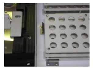
Pay attention the direction of reagent shelf load, and make sure to place the shelf balance touch with the bottom .
