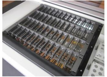
(3). Put some water on every slides and observe whether its stay in the slides over two-thirds, the slides position is slightly slope forward, if not, please adjust the six feet of equipment.
