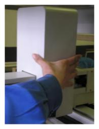
(3) Cut off the tape for the left/right pillar and take away the pillars, try to pull the beam. (See figure b)
