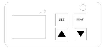
SET--- This function is used to set the temperature. Press the button, and the indicator lamp will
