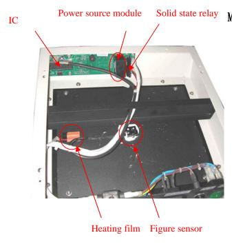
Maintenance: Use Philip screwdriver to loosen the six screw in the base-plate, and take down the base-plate, and there will be a power source module on the main board in the instrument as it shows on the picture. And take down the power source module from the main board by hand, if it is difficult to take down the power source module with hand, you can use the flat apparatus as flat tip
